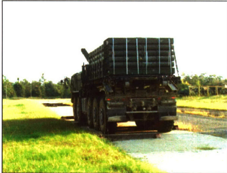
Photo 9. Hazard Course Testing of the LVSR
