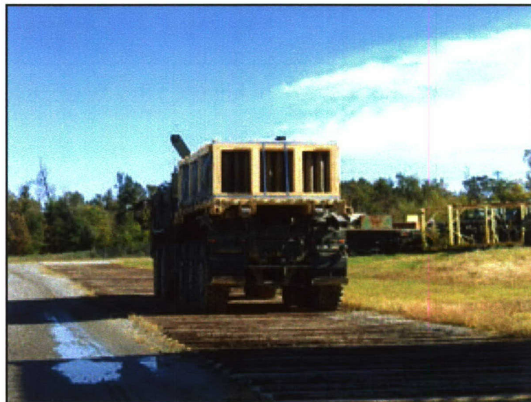
Photo 24. Washboard Course Testing of the LVSR
