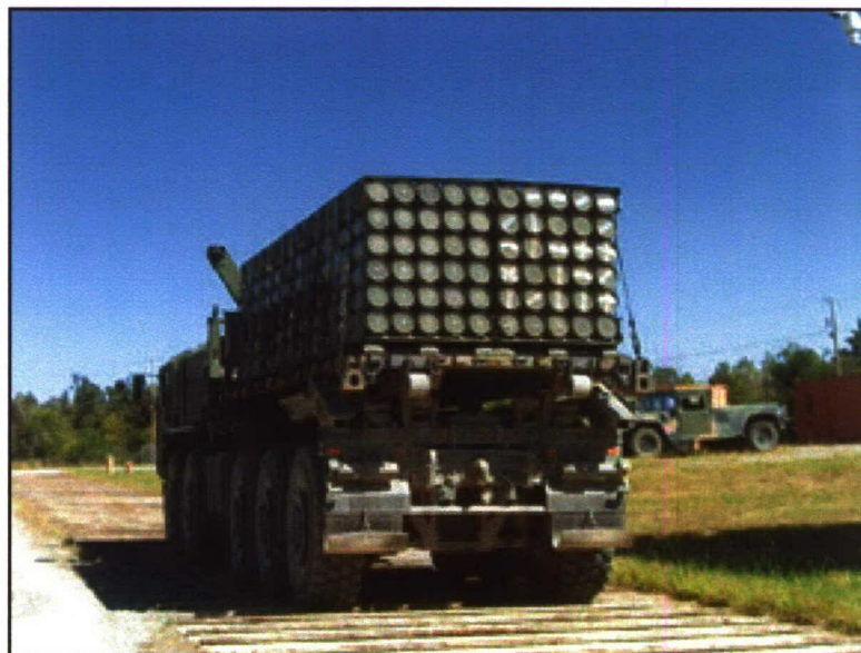
Photo 17. Washboard Course Testing of the LVSR.
