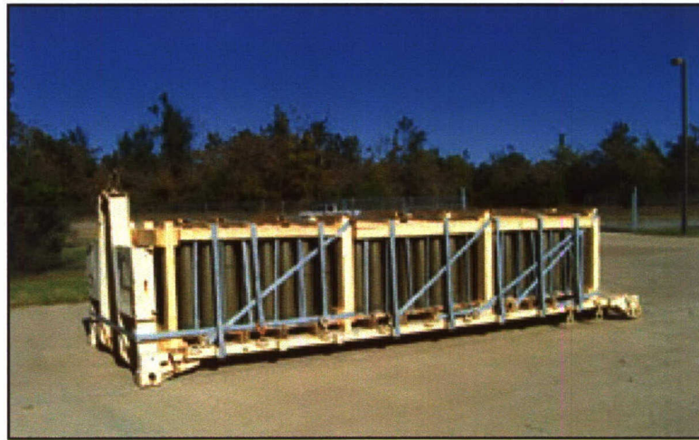
Photo 21. Flatrack Loaded with 155MM SLPs Secured with Steel Banding.
