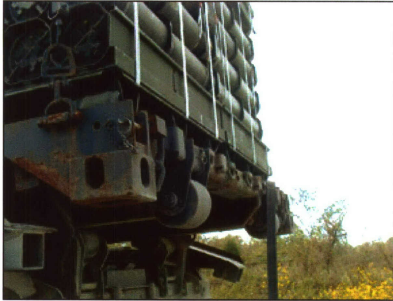
Photo 11. Sheared Bottom Strap.
