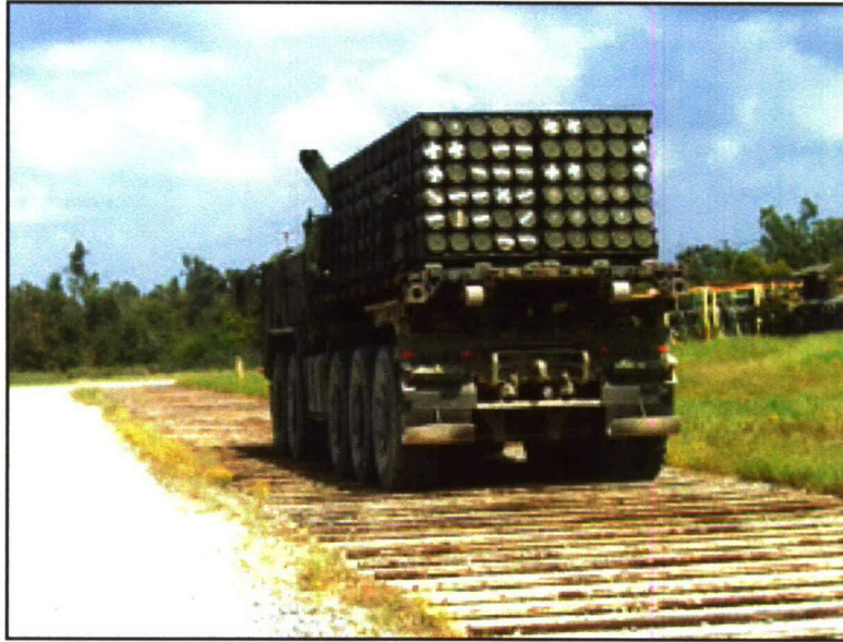
Photo 7. Washboard Course Testing of the LVSR.
