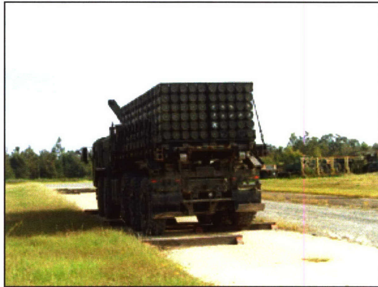
Photo 13. Hazard Course Testing of the LVSR
