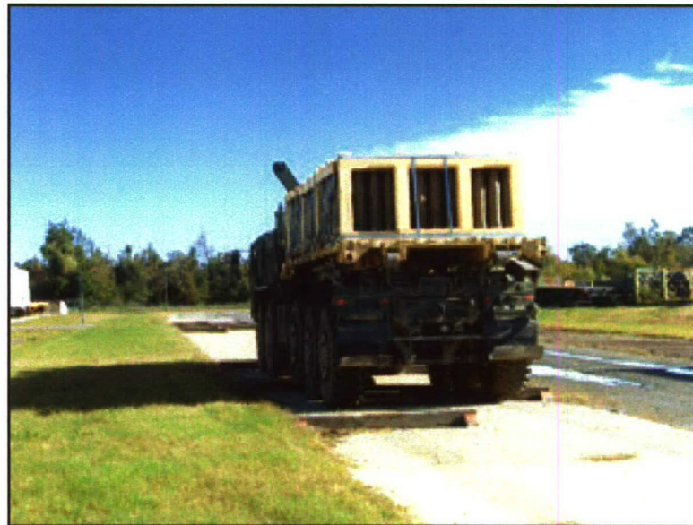
Photo 23. Hazard Course Testing of the LVSR.
