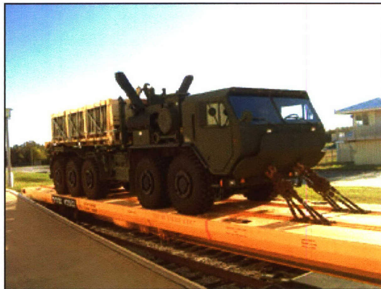
Photo 22. Rail Impact Testing of the LVSR (Prior to Testing).
