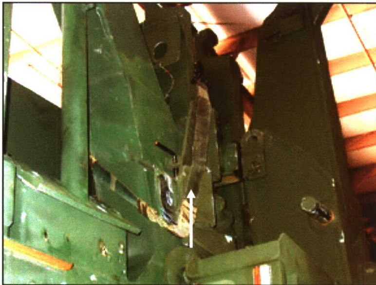
Photo 3. Strap Holding Flipper Arms
