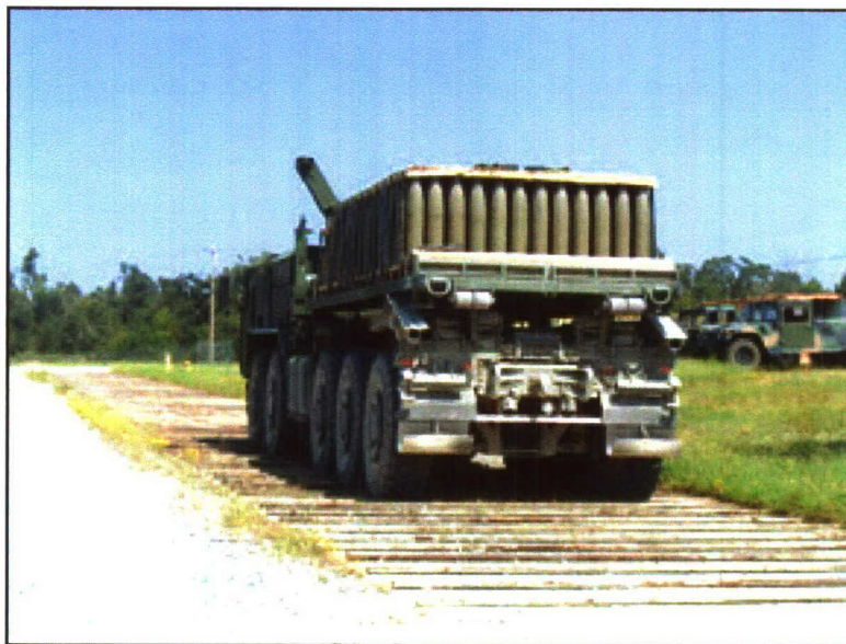
Photo 20. Washboard Course Testing of the LVSR.
