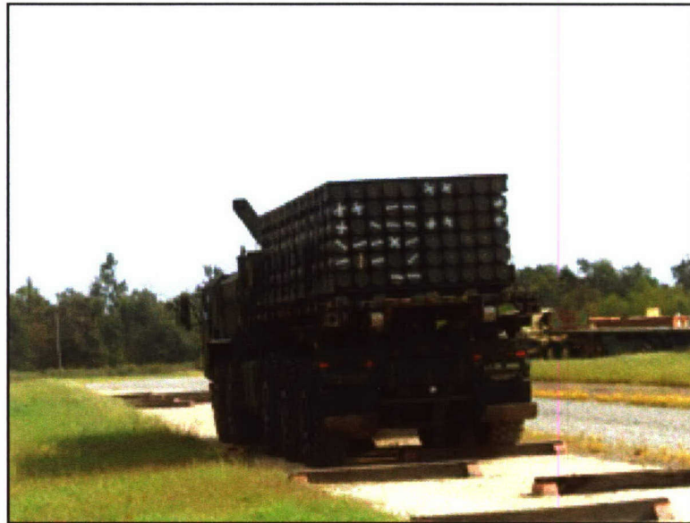
Photo 4. Hazard Course Testing of the LVSR
