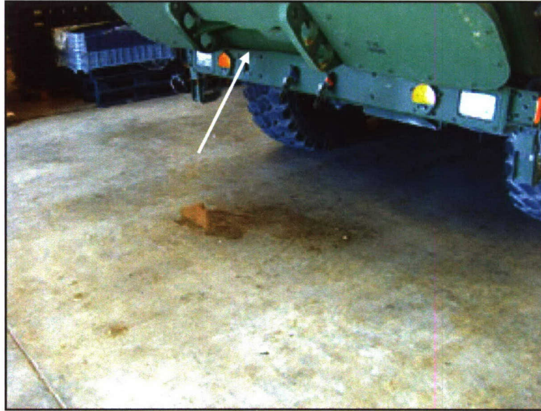
Photo 26. Coolant Leakage Point.
