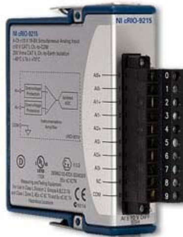
Figure 55. NI cRIO-9215 Analog Input Module. From [32].
