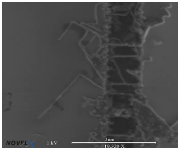
Figure 8. Si wires bridging the trenches.
