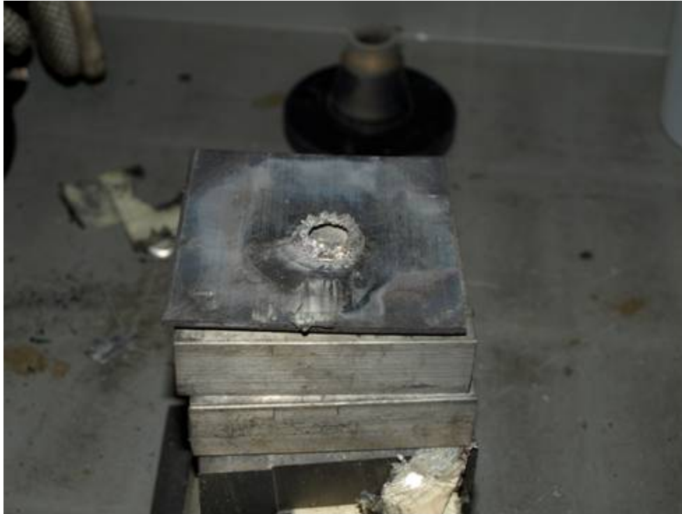
Figure 47. Damage to top target plate: Test 2-3.
