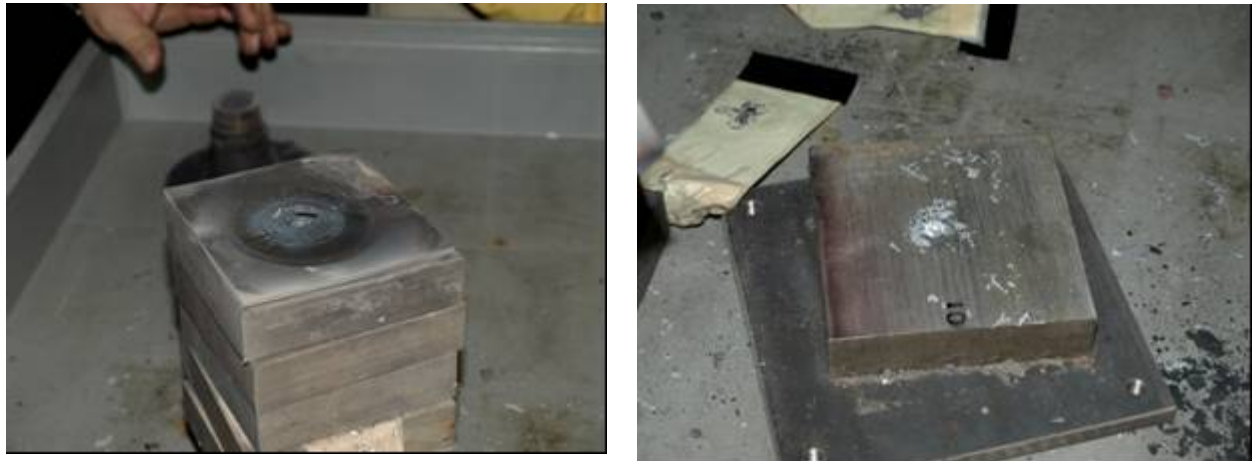
Figure 50. Jet penetration through first and last target plates: Test 2-6.
