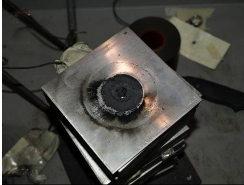
Figure 35. Damage to top target plate: Test 1-1.
