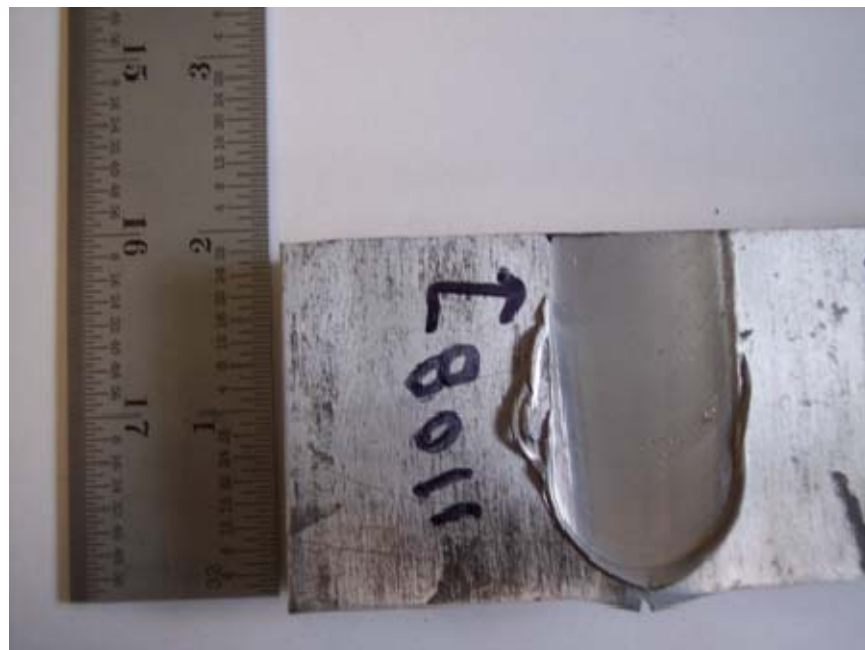
Figure 2. Result of FSW on Al-Li Alloy
