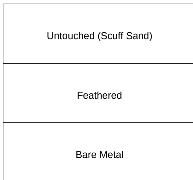
FIGURE 14 – Schematic of the 12”x12” panel used for evaluating the reparability of the Mg-rich primer coating system.
