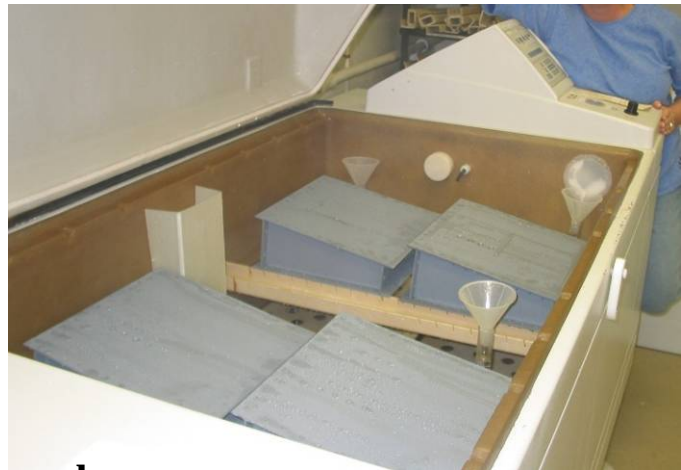
FIGURE 5 – a.) SAS box surface panel with each column of different fasteners identified (A: Steel Jo-Bolt, B: Ni/Steel Blind Rivet, C: Aluminum Blind Rivet, D: Aluminum HI-LOK ® , E: Steel HI-LOK ® ), and b.) SAS boxes being evaluated in ASTM B 117 salt fog.
