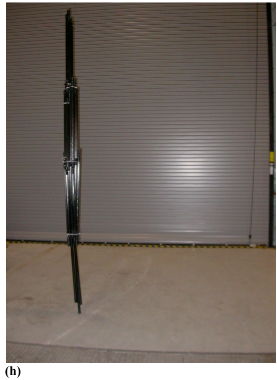
Fig. 2 Four-captured MACSES reconfiguration events depict an abbreviated three-bay model and prototype at each stage of the sequence, (a,b) (i) an expanded truss bay disposed between two-, expanded hub bays, (c,d) (ii) the truss bay sheared to collapse this assembly against the faces of the hub bays, (e,f) (iii) the first hub bay shear substantially collapsing the structure into a planar topology, (g,h) and (iv) the last stage, the simultaneous second hub bay shear and the second truss bay shear substantially collapsing the structure into a linear topology.
