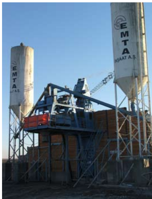
Concrete batch plant to mix concrete
