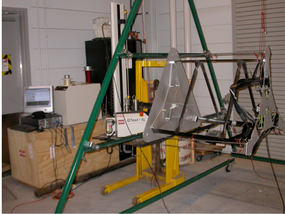
Fig. 4 Measurement of the deployment force profile, developed by the passively sequenced, 450 mm radius, 30.0° diagonal angle, and three-longeron DECSMAR test article, was sought by fixedly attaching a 1.33 kN capacity load cell, rated at 0.08% full scale precision, to the out-board endplate of the boom. The article was mounted normal to gravity at the in-board endplate and the load cell, out-board endplate, and cantilevered structure were off-loaded from a trolley constrained to a track parallel to the primary structural axis.
