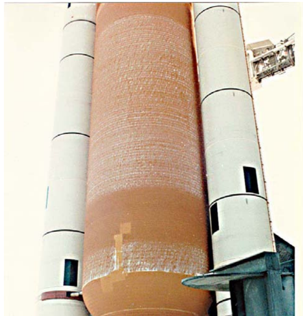
Figure 1. Ice/frost formed on an ET
