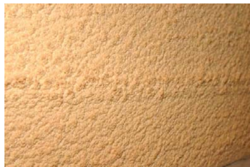
Figure 4. A section of ET SOFI showing its roughness
