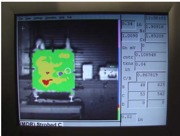
Figure 20. Thin shell ice balls of 2 in. (in red) and 3 in. diameters (in blue) detected at 25 ft. and 90 degrees (right)
