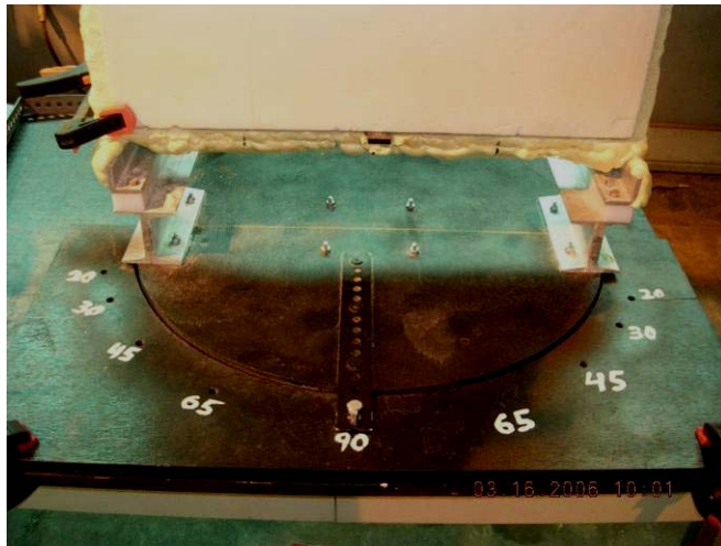
Figure 6-4. Turntable with CTC mounted on top in 90-degree position
