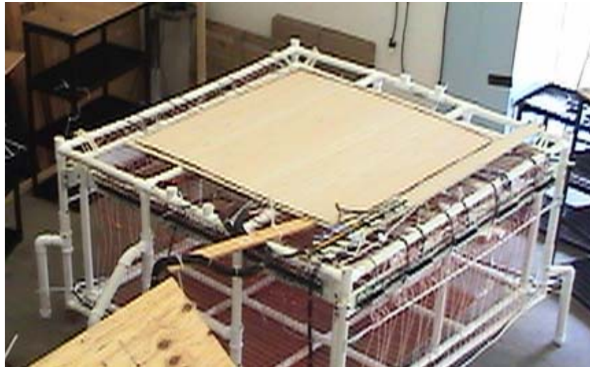
Figure 47 Top view of secondary differential Z-receiver coils
