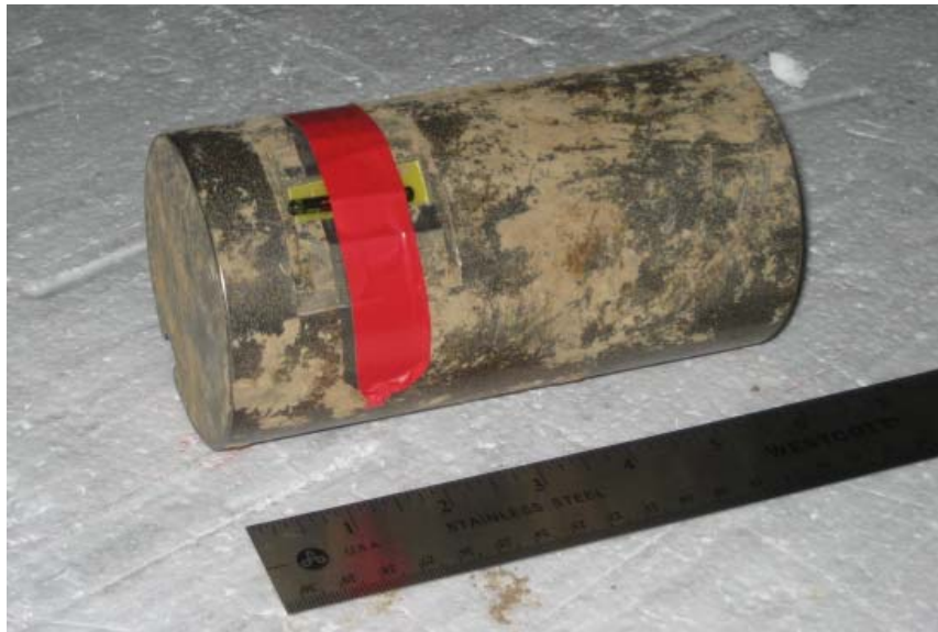
Figure 70. Munition surrogate later buried at Aberdeen Test Center. The tag is evident below the red tape.
