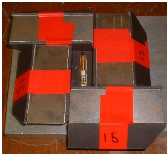
Figure 86. Test configuration including the Tiris transponder and four pieces of carbon steel used to simulate the tag embedded in a munition. The walls are at 90° in this photograph.
