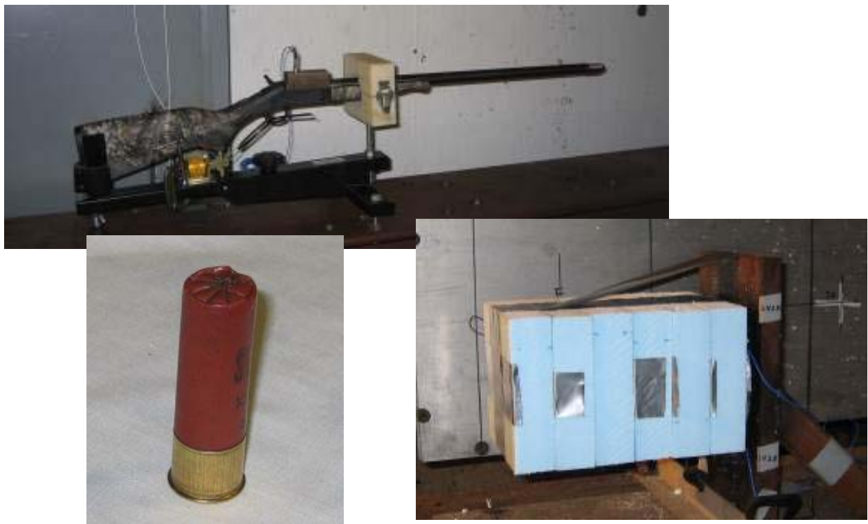
Figure 68. Setup of the firing tests at West Jefferson showing the shotgun, the shotgun shell containing the tag, and the Styrofoam fixture for the soft catch of the test slug
