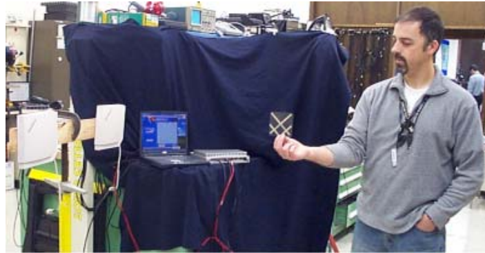
Figure 53. Laboratory setup of range and azimuth measurements with the Matrics tag
