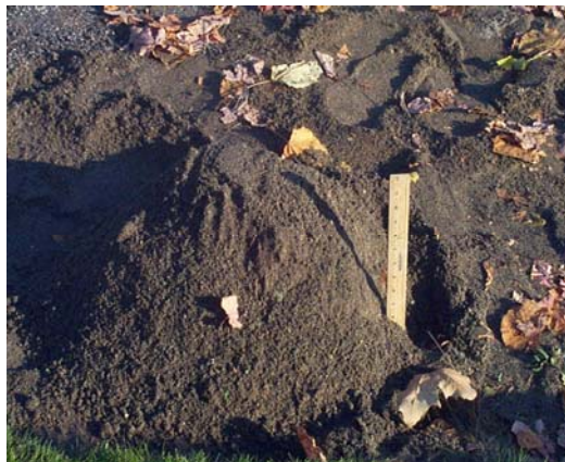
Figure 44. Mounding of soil to achieve greater overburden thickness.
