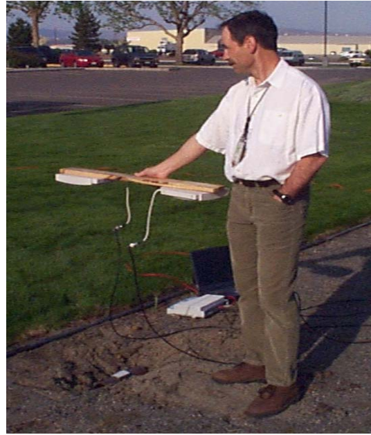
Antennas Perpendicular to the Munition Length
