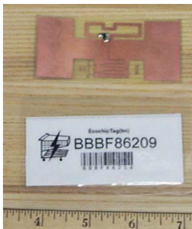
Figure 45. Trolley Scan UHF tags; naked tag (above); tag in plastic laminate (below)
