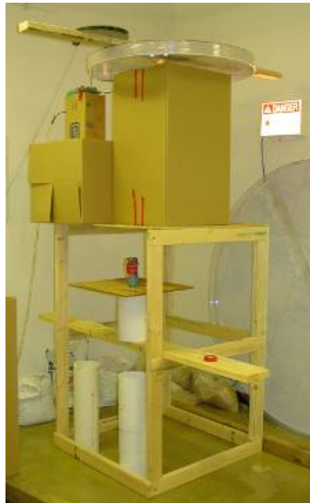
Figure 32. Laboratory setup for characterizing the one-meter transmit coil and the Tiris tags
