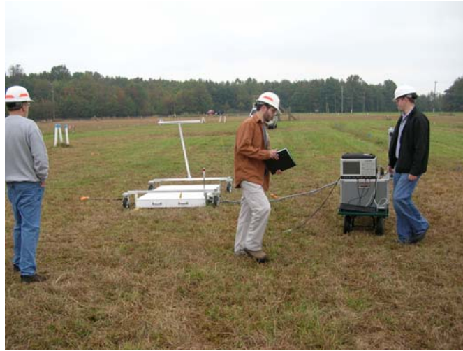
Figure 79. Coil module and electronics module being used at Aberdeen Test Center in 2006
