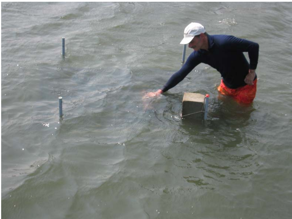
Figure 14. We collected data with the indexed platform immersed in seawater, with the sensor fixed to the frame underneath the target grid; a target jig that slid along indexed rails facilitated positioning. The larger targets required deeper (higher tide) water than shown.
