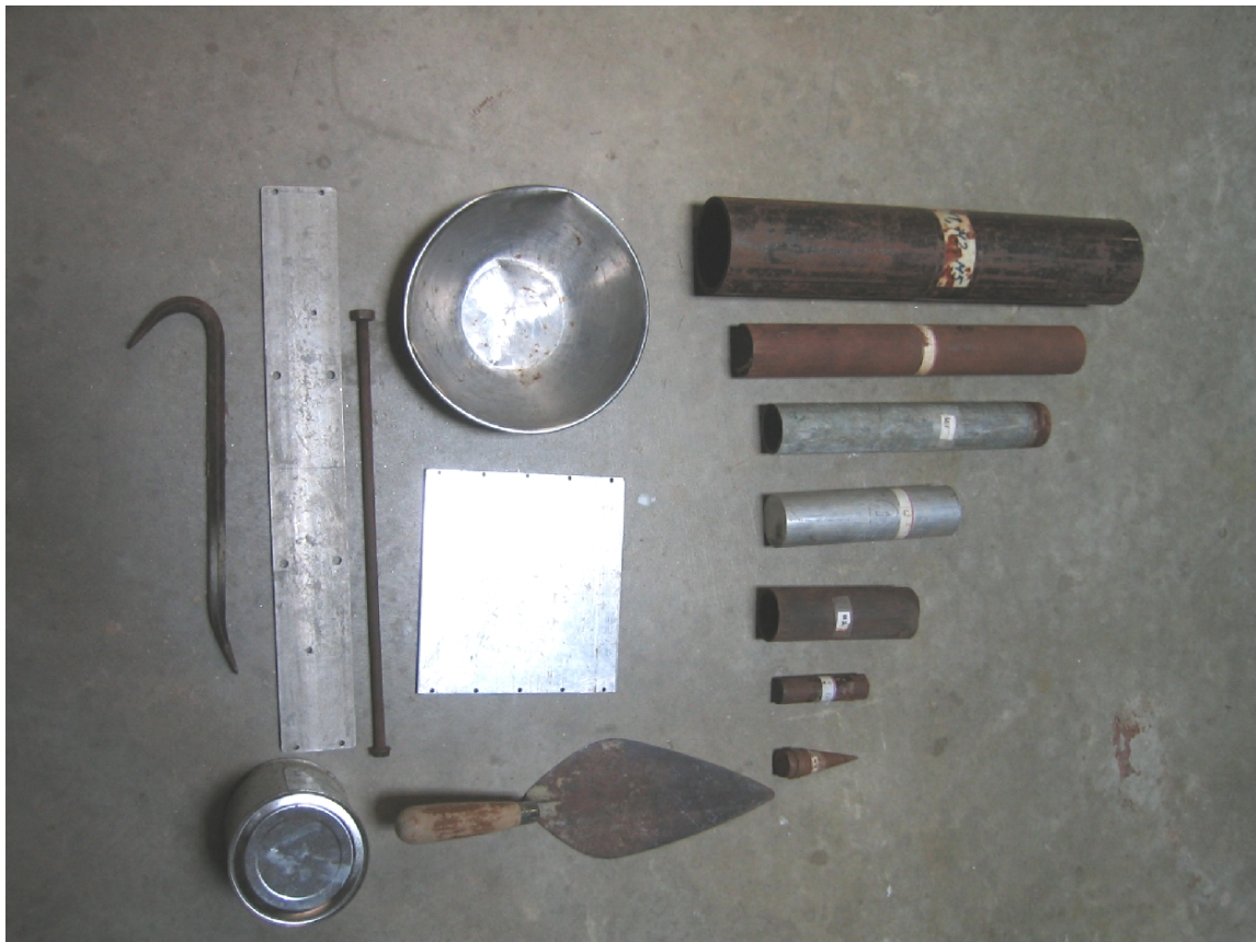
Figure 4. Targets used for the discrimination experiment, with seven surrogate UXO covering a wide range in size (right side of photo), and seven clutter items of various form.
