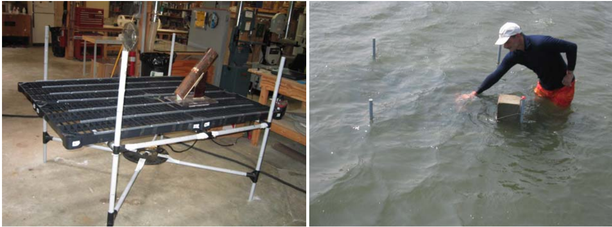
Figure 3. Final experimental setup showing the GEM-3 mounted on the frame below a target mounted on a jig that fit on rails with positioning slots in air (left), and in water (right), providing precise target-sensor geometry control over a 2-dimensional grid.
