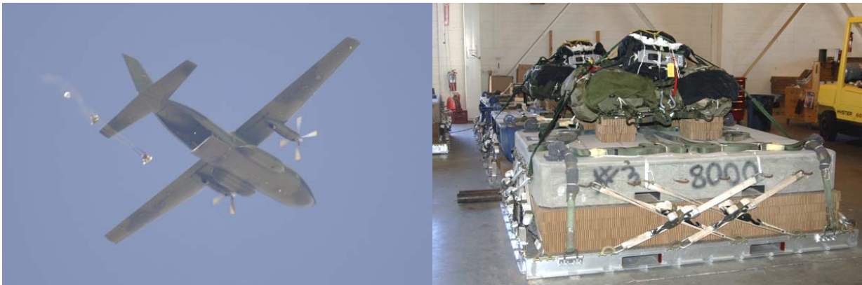
Figure 6: PAD system drop from C-160 Transall aircraft (left) and heavy PAD system rigged for airdrop (right) at PATCAD
