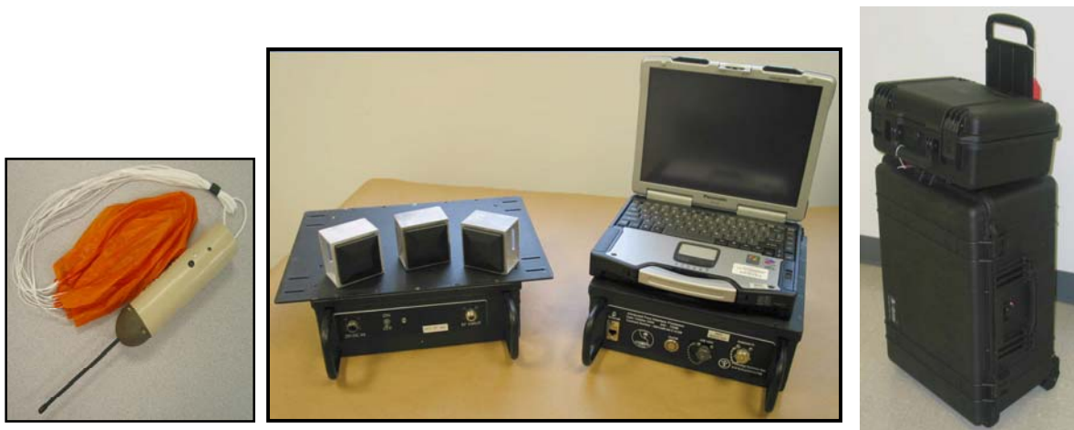
Figure 1: JPADS-MP Fly-Away Kit. (From left to right: Dropsonde, JPADS-MP Hardware, Laptop, and Carrying Case)
