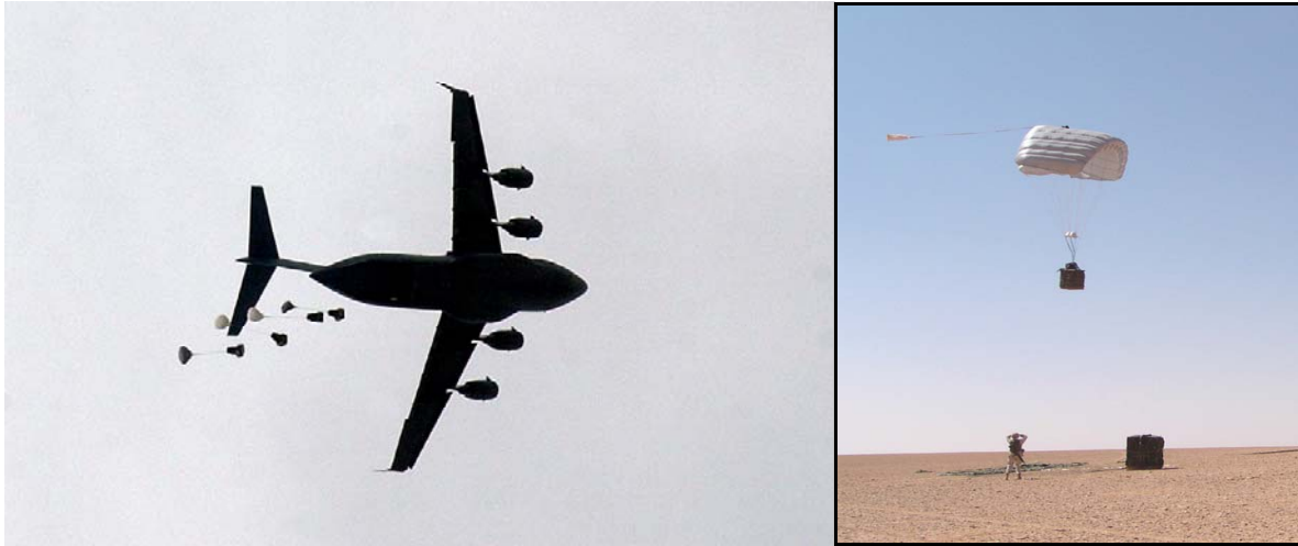
Figure 3: Four Sherpas shown exiting C-17A aircraft (left) and just prior to landing (right).
