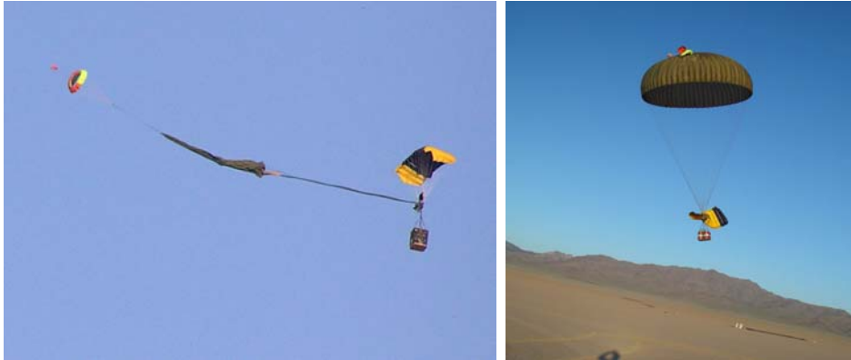
Figure 4: JPAD-XL SCREAMER transition from guided flight (left) to recovery chute landing (right).
