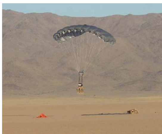
Figure 1 (left) Release of 500 kg payload with SPADES using the Firefly parafoil of Para-Flite
