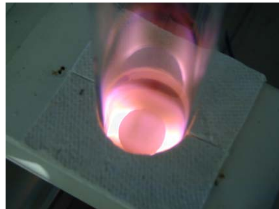
Figure 1: Experimental set-up MESOX with the irradiated shutter (top, right) placed at the focus of the 6 kW solar furnace (top, left). Images of plasma environment: CO 2 (down, left) and air (down, right).
