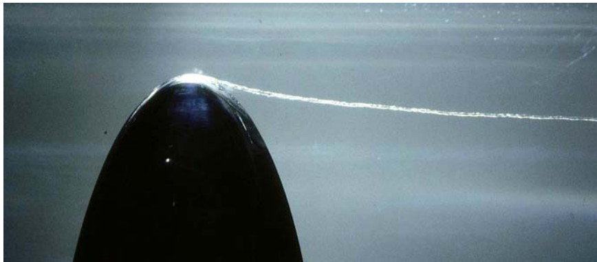
Figure 6: Vortex Cavitation Generated by a Three-Dimensional Hydrofoil.
