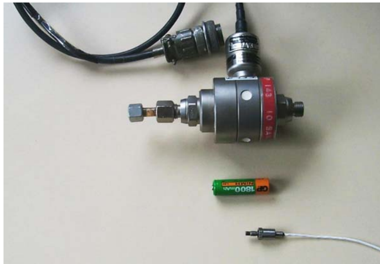
Figure 4: Pressure Sensors with Four-Arm (Wheatstone) Bridge for Steady (LUCAS SCAEVITZ, top) and Unsteady (KULITE, bottom) Pressure Measurements. Battery (middle) to compare size.
