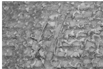
Fig. 46 Mounted TC 7 and 10 on ablator surface
