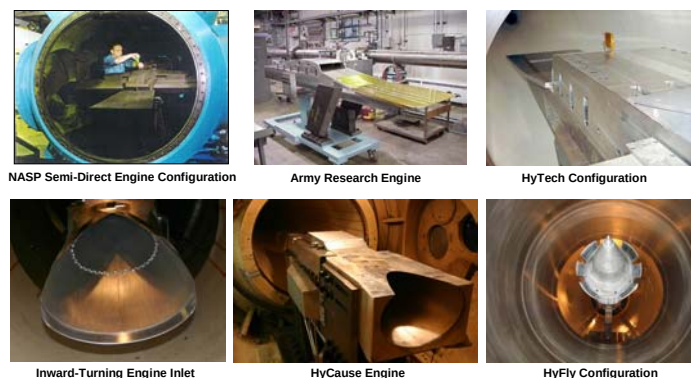
Figure 62: Scramjet Engines Tested in LENS Facility
