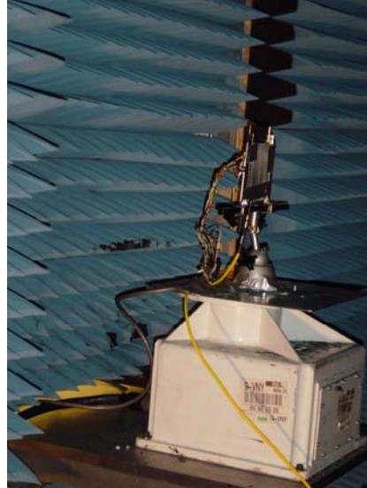
Figure 8. MEMS ESA attached to rotary stage within anechoic chamber at AMRDEC.
