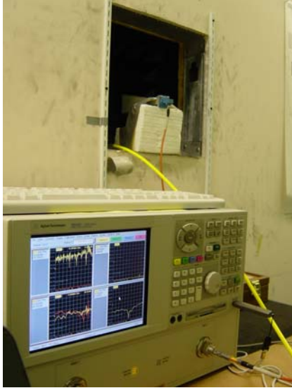
Figure 7. Horn antenna connected to Agilent PNA-L network analyzer at far end of AMRDEC's anechoic chamber.
