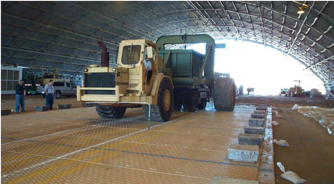
Photo 29. DURA-BASE® Being Subjected to Traffic on the SM Test Section
