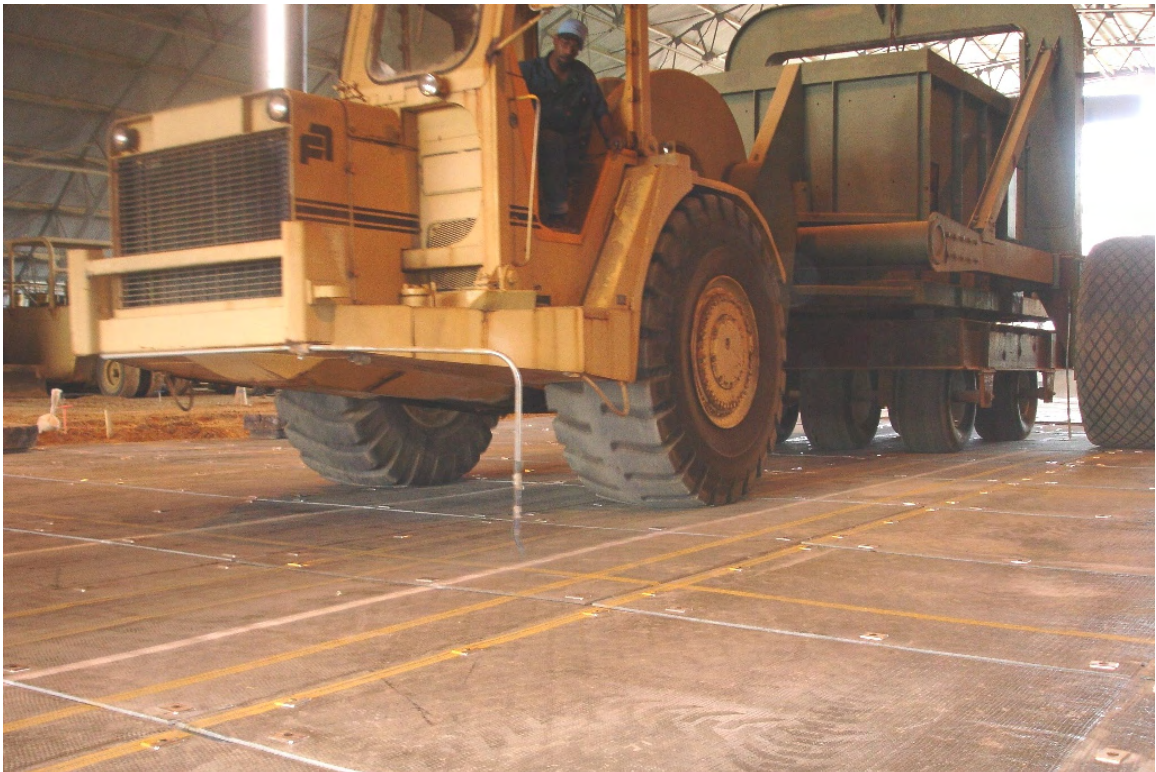
Photo 30. Trafficking of C-17 Full Gear Load Cart on ACE-Mat™ Placed on SM Test Section
