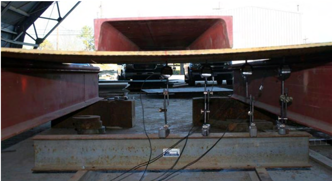
Photo 34. Composite Modulus Testing on ACE-Mat™. The Loading Beam is Placed on Top. Note the 4 Deflection Gauges Below. The Mat was not Deflected before Placement of the Loading Beam, which was included in the Deflection Weight
