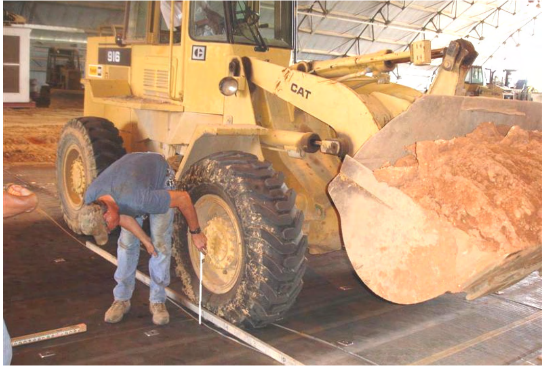
Photo 25. Using Loaded Front-End Loader to Load the Mat for a True Deformation (Rut) Measure
