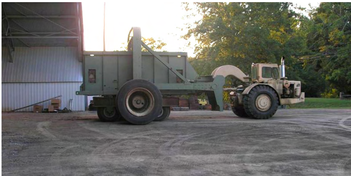
Photo 24. C-17 Load Cart (C-17 Mock Gear Set is Behind Large Outrigger Tire)
