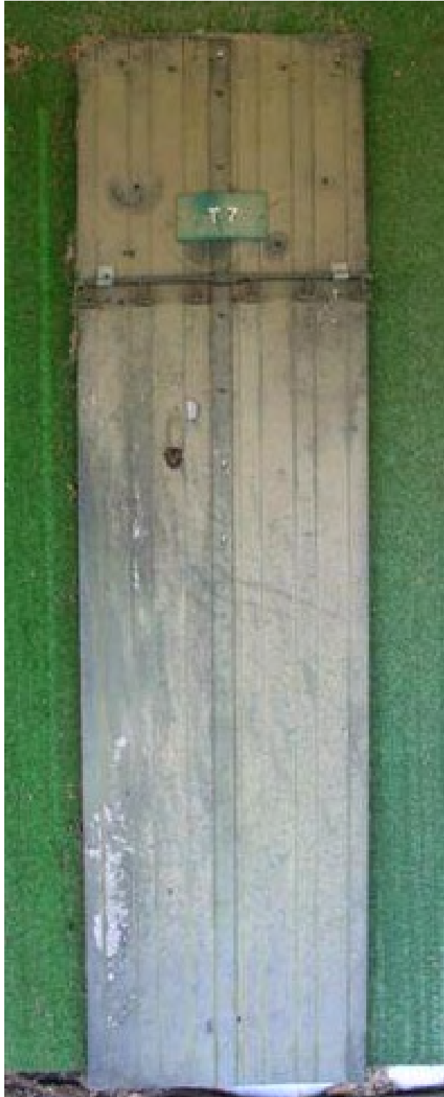
Photo 4. T7 mat, note the cross section bolted under the mat label
