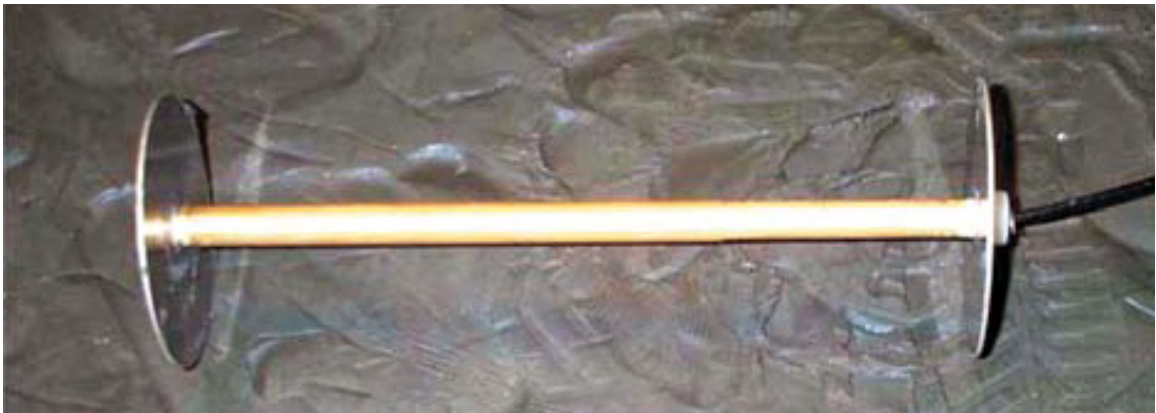
Photo 23. Soil Compression Gauge by CTL Group
