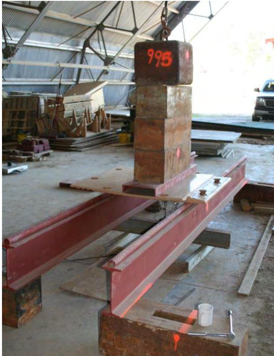
Photo 35. The Composite Modulus Testing on Bravo® Mat. Note this Load is Approximately 1,270 kg (2,800 lb)
