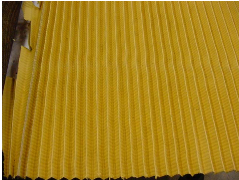
Figure 15. Test Elements from Environmental Tests—Inner Side of Pleated Media
