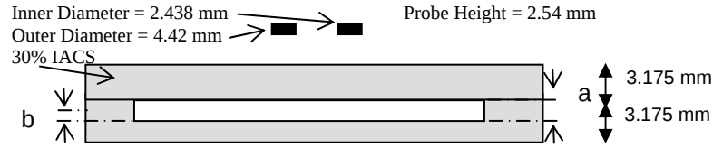
Figure 1. Diagram of two layer system with material loss at the faying surface.
