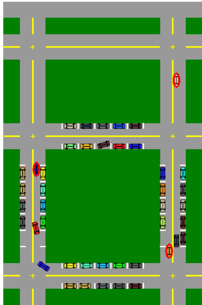
Figure 6.34: A later snapshot taken at 31.33 seconds during the simulation. In this figure, cars surrounded by red ellipses are cars that are stopping due to the ‘Hazard’ input signaled by the timed stop-light.
