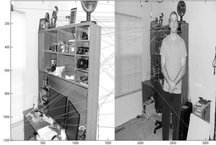
Figure 4.9: SURF Image Showing Reduced Keypoint Matches With Occlusion.
