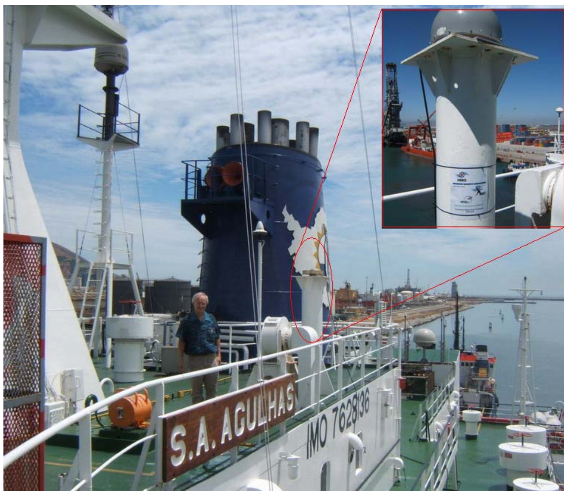
Figure 7: Location of the GPS choke ring antenna on board the SA Agulhas. Inset shows antenna with radome.
