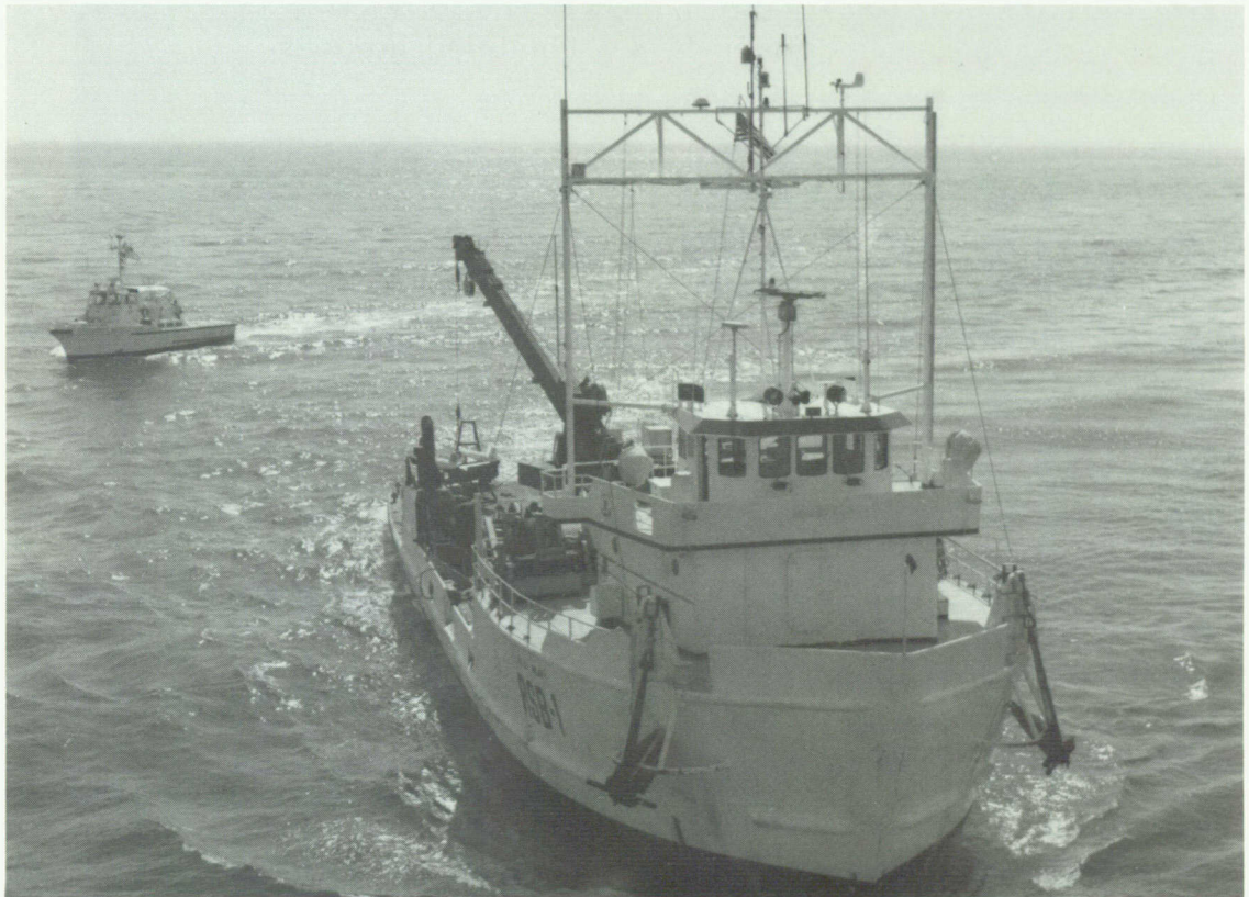
The deck of the 195-gross-ton RSB-1 forms a 2900-square-foot work area.
