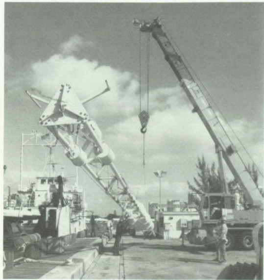
Forty-ton crane lifts APL heat flux spar buoy to deck of RSB-1.
