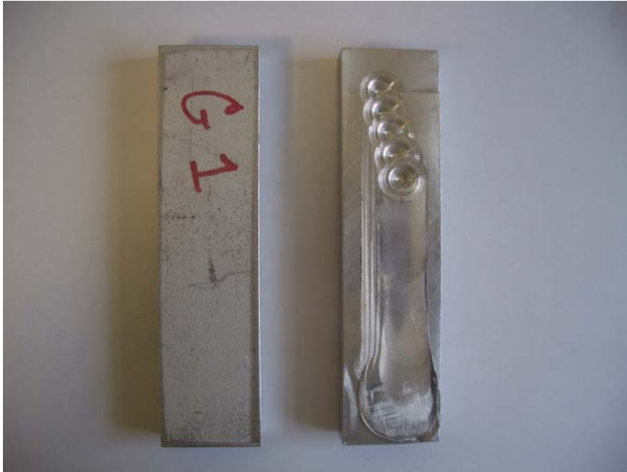
Figure 4. Image of AA5083 G1 material in the as-cast condition compared to the material following multi-pass FSP.
