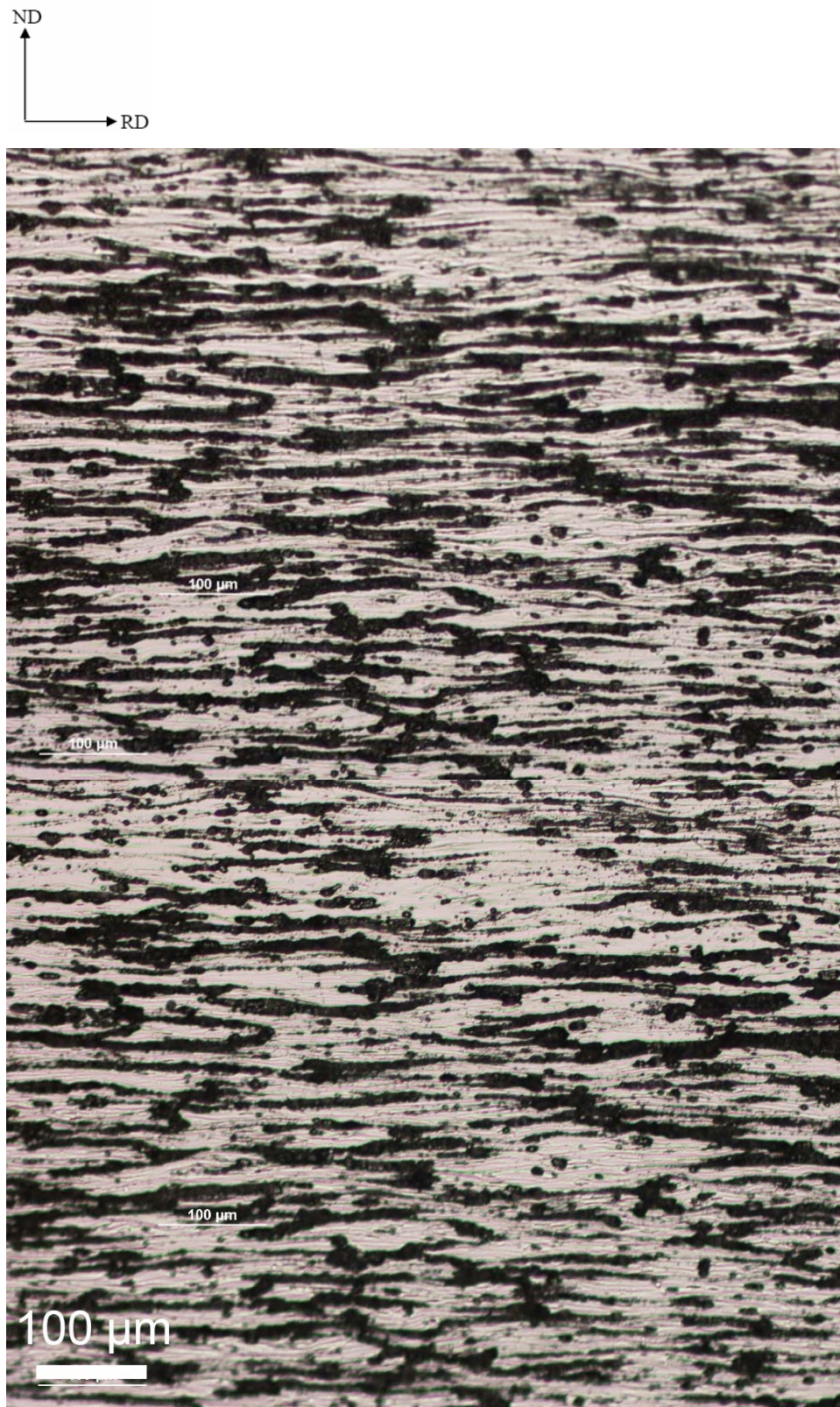
Figure 7. Optical microscopy of received HB AA5083 showing elongated grains having widths between 20 -120 \mu\text{m} .
