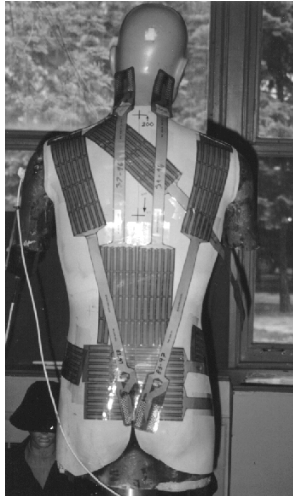
Figure 2 LC Simulator mannikin, with F-Scan™ pressure sensors in place.
