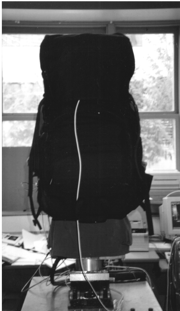
Figure 2.1.1. Photograph of CTS Prototype Pack K1 positioned on LC simulator mannikin
