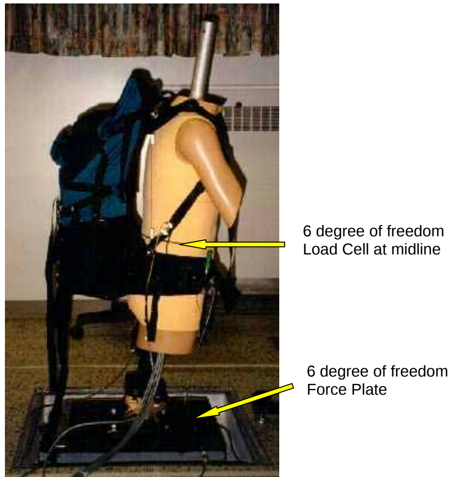
Figure 2. Load Distribution Tester
