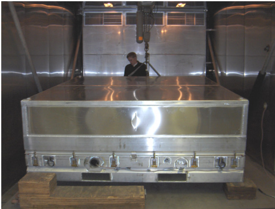
Figure 12. Rotational Edge Drop (+60°C).
