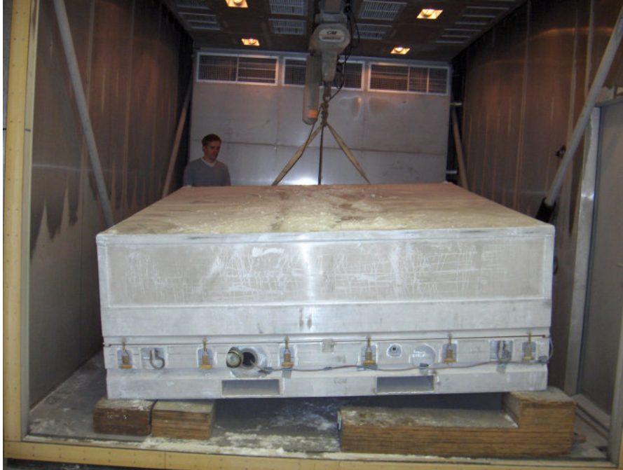
Figure 11. Rotational Corner Drop (-40°C).
