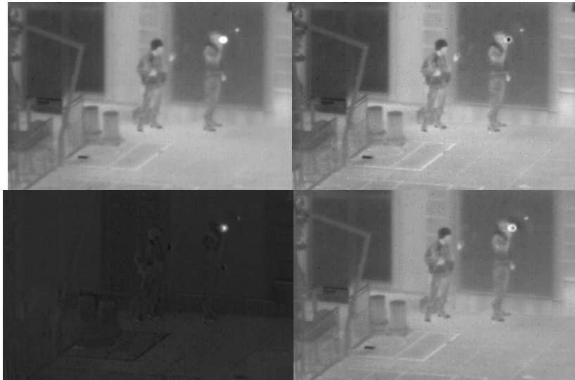
Figure 3-13, clockwise from top left: MWIR, LWIR, opponent fused, DWT fused to scale 4
