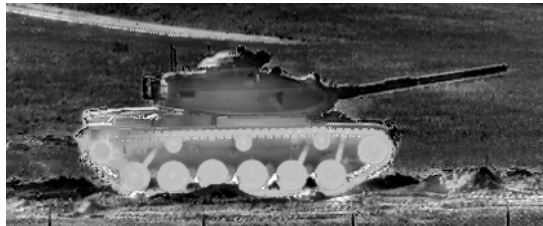
Figure 11: Laplacian A image fusion
