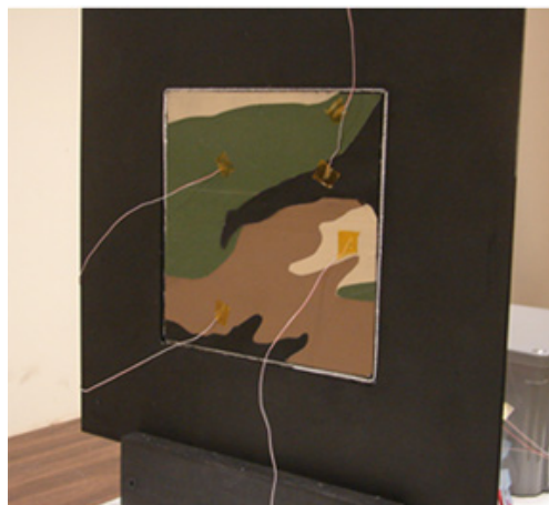
Figure 6-2 Aluminum plate with woodland camouflage pattern formed with flat black paint and low-emissivity tape.
