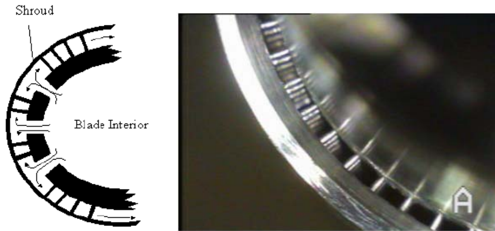
Figure 4. Cross section of heat exchanger in stainless steel tube [from Marques, 2002]
