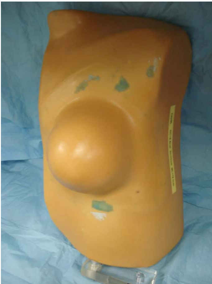
Figure 1: Compressible and deformable breast phantom
