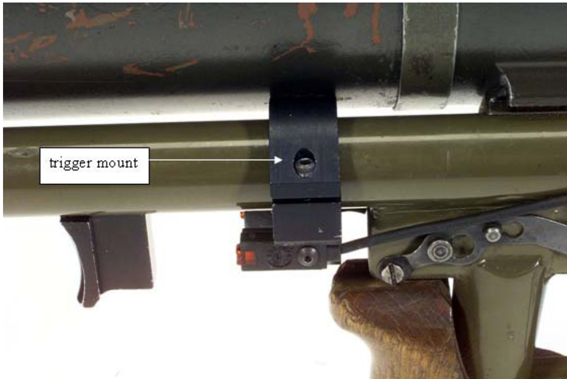
Figure 1: SAT sensor Trigger Mount correctly installed
