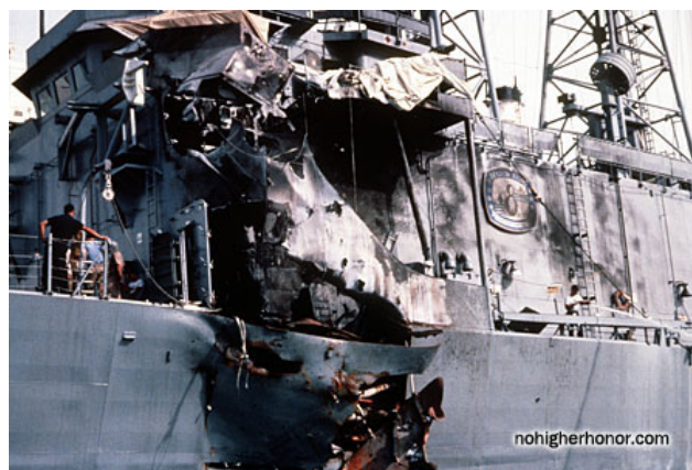
Figure 3-5. External view of the damage caused to the USS Stark by two Iraqi Exocet missiles.
