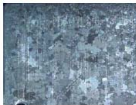
Figure 11: MIL-PRF-46170 (Cadmium - corrosion at 135°C)
