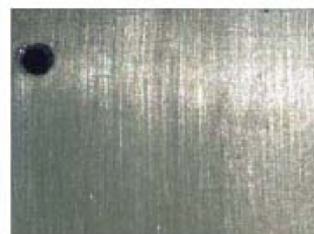
Figure 9: MIL-PRF-2104 10W (Cadmium - tan colored at 135°C)
