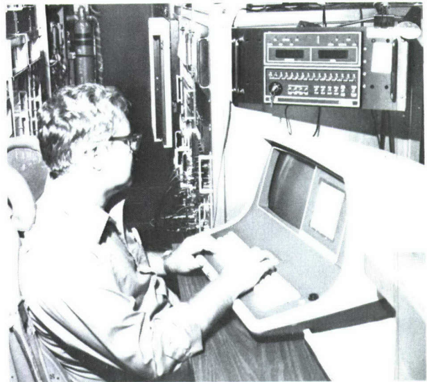
Figure 3. William H. Hopkins manning the operator control station in the EP-3A flying laboratory, showing instrumentation, computer, and magnetic tape recorder
