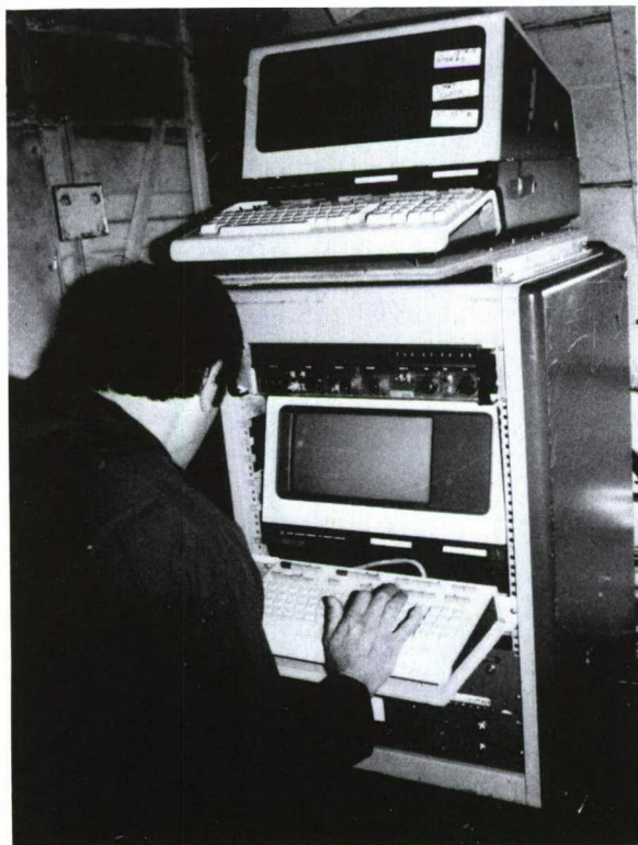
Figure 14. Daniel Steiger at the console of AXBT data acquisition and processing system aboard an NRL aircraft
