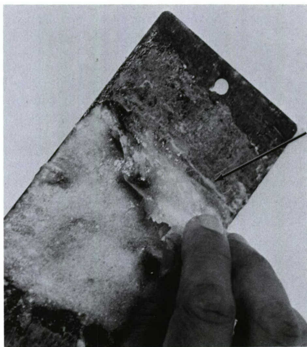
Figure 3. Removing the cleaning strip that contains the rust and other corrosion products
