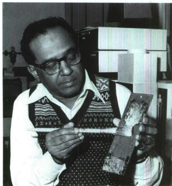
Figure 1. Dr. Panayappan applying the PVP/EDTA cleaning formulation to a typical rusty surface
