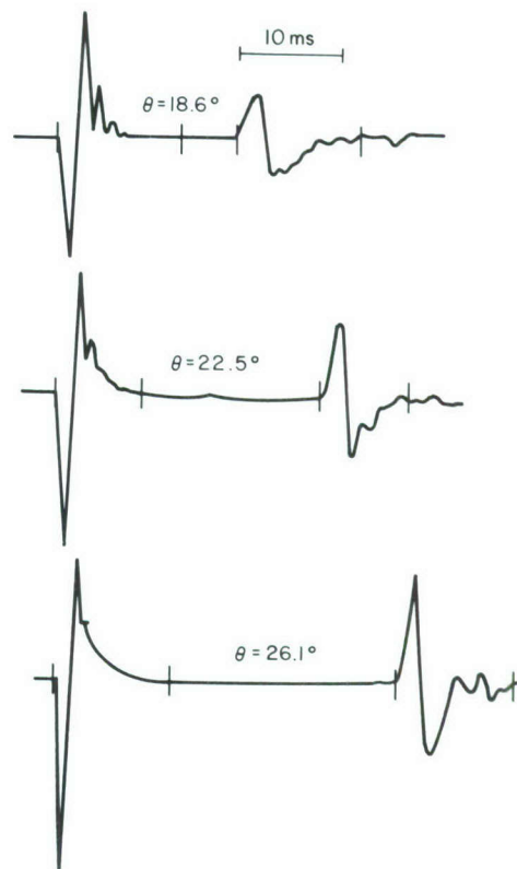
Figure 4. Pressure vs time series of direct and ice-reflected arrivals. The pulses used for FFT are between the vertical bars.
