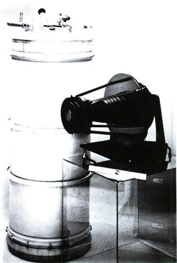
Figure 5. The FIRSSE dewar and telescope. The dewar keeps the optics and detectors at cryogenic temperature (liquid helium). The cover, shown here at the bottom of the dewar, is removed above the atmosphere and is replaced before re-entry. The telescope is a folded Gregorian system of all-beryllium construction.
