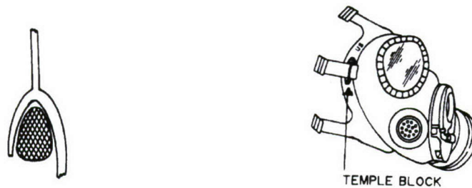
Figure 8. Location of Foam Inserts Integrated into Mask Prototypes (Stark et al., 1988)
