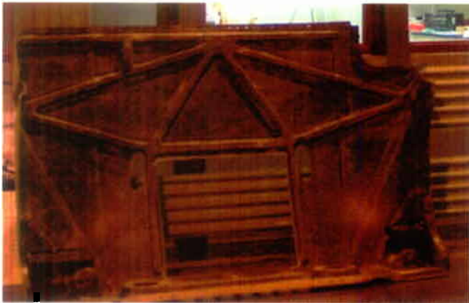
Figure 10: HMMWV Composite Hood
