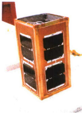
Figure 1. Photograph of the PSSC engineering development spacecraft body.
