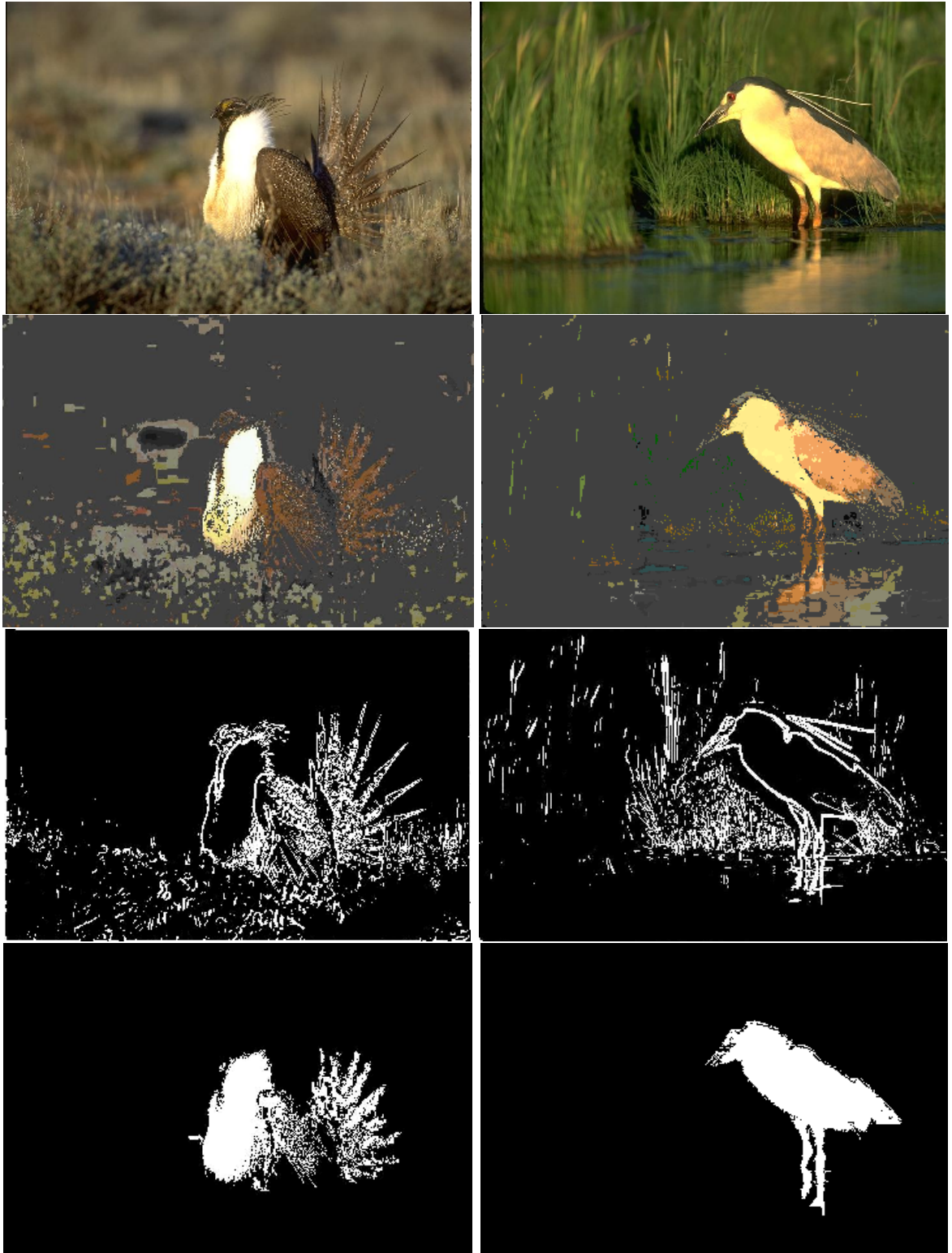
Figure 5.8. Examples of region of interest segmentation : (row 1) original images (row 2) remaining image after background colors are eliminated (row 3) edge image (row 4) final segment obtained
