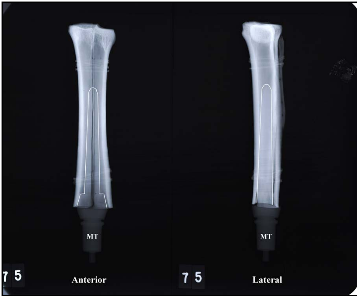
Figure 7. Anterior and lateral radiographs of metatarsal III with Delrin trial implant inserted. The Delrin implants have been outlined in white for easier viewing. MT = Morse Tapered post for prosthetic attachment.
