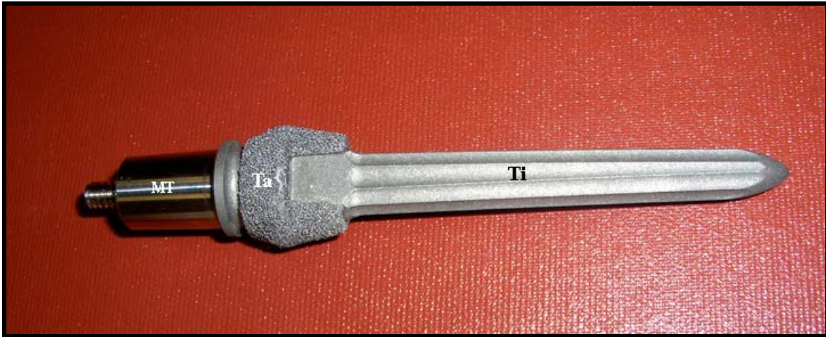
Figure 8. Image of titanium (Ti) and tantalum (Ta) implant. Design features include a Morse Taper (MT) where the prosthesis will attach, a region of porous coating (Ta) where bone ingrowth is to occur, and a fluted and grit blasted titanium stem (Ti) for endosteal attachment and rotational stability.
