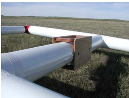
Figure 5. ORAGS-EM Small Loop Receiver Coil Configuration. (Inset shows enlarged view of coils.)
