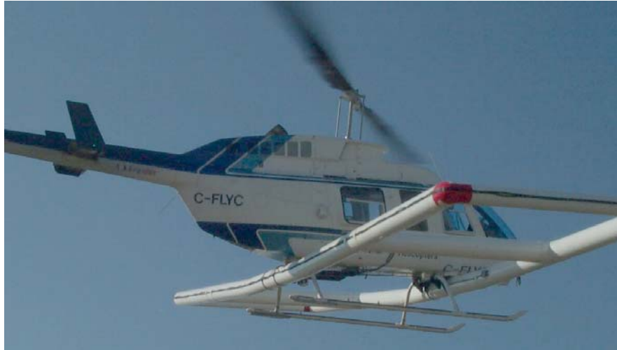
Figure 4. ORAGS-TEM Large Receiver Loop Configuration. (Single loops of wire are attached to the top and bottom of the 3m x 3m outer portion of the booms to form the large-loop gradient receiver.)
