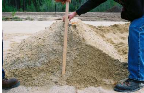
Figure A-20: Lane End Berm from HLS Front Scoop
