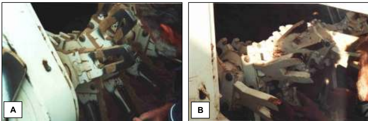
Figure 6: MCC Auger Fingers: Straight (A) and Twisted (B)
