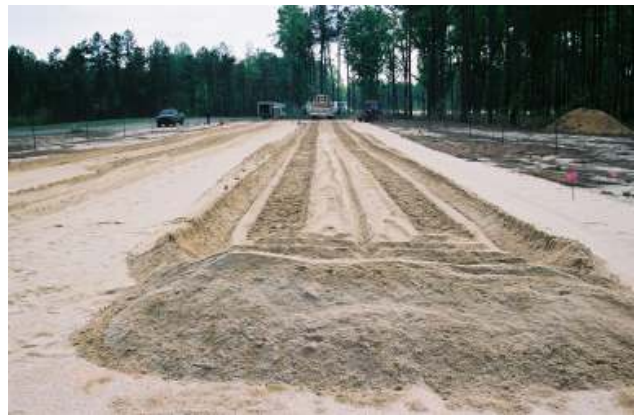
Figure A-12: Sifted Sand Lane with End-Berm
