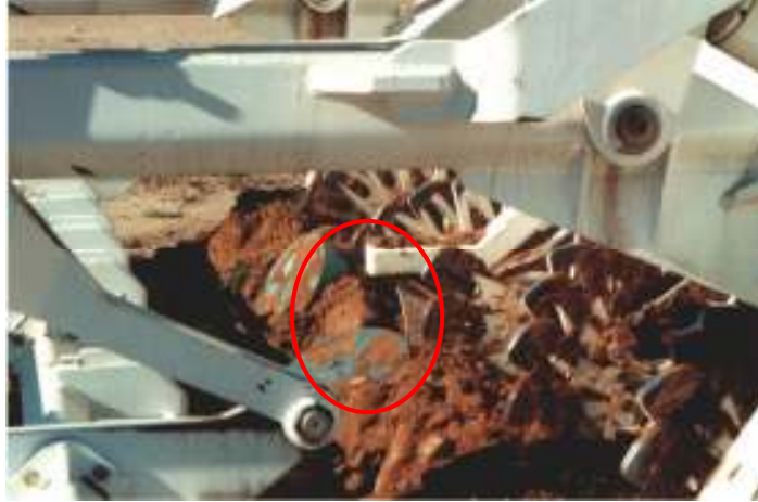
Figure 25: Mine Caught Under Center Bar
