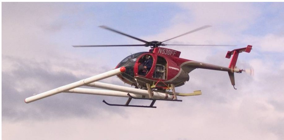
Figure 2. Sky Research, Inc. MD 530F helicopter and magnetometer boom assembly. Seven magnetometers are contained in the composite-material boom and positioned with the GPS antenna and laser / acoustics altimeters.
