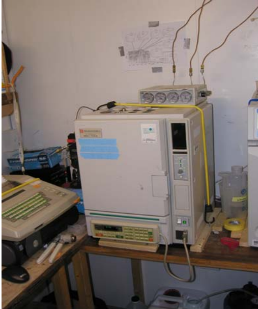
Figure 9: Shimadzu GC 14A used for porewater methane analysis.
