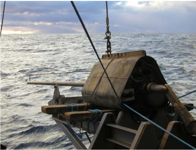
Figure 12: Sediment heatflow “Lister-type” system deployment.
