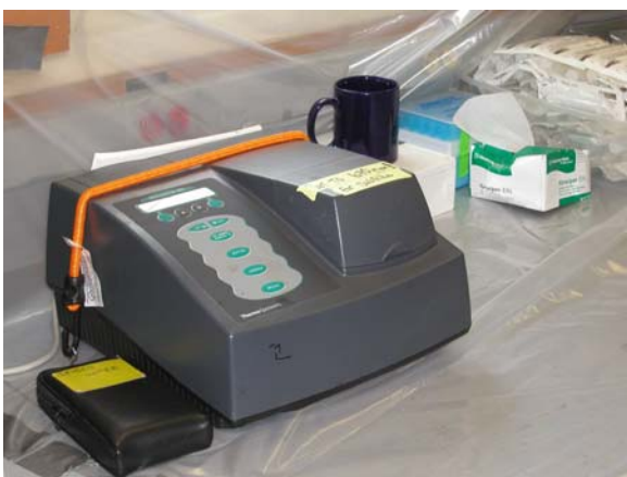
Figure 10: ThermoSpectronic Genesis 20 spectrophotometer used for porewater sulfide analysis.
