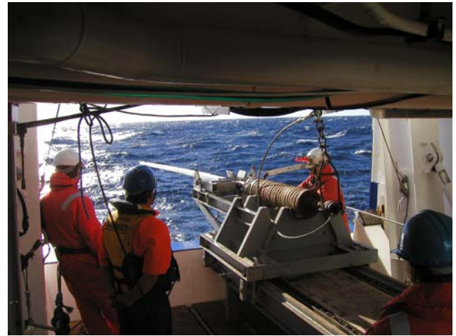
Figure 6: Piston coring system provided by NIWA.
